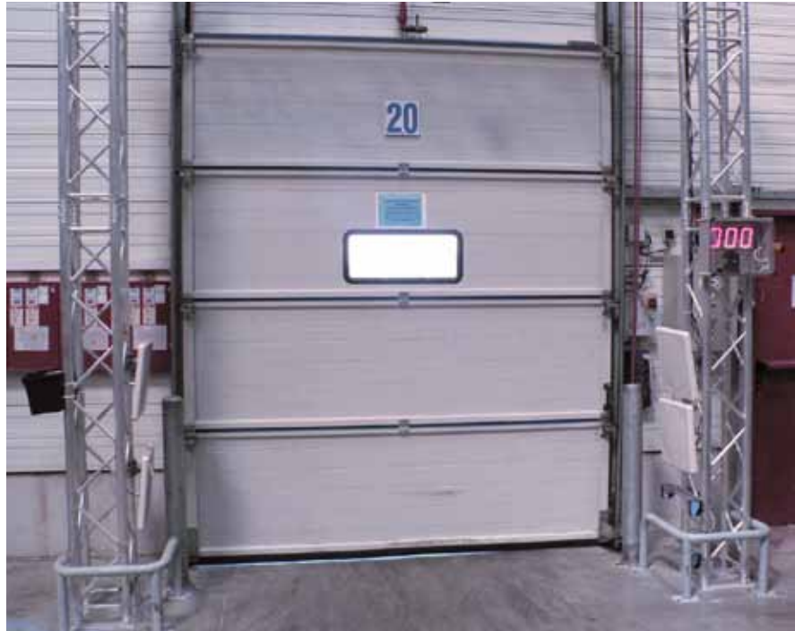
RFID portal deployed during the pilot at Carrefour warehouse
