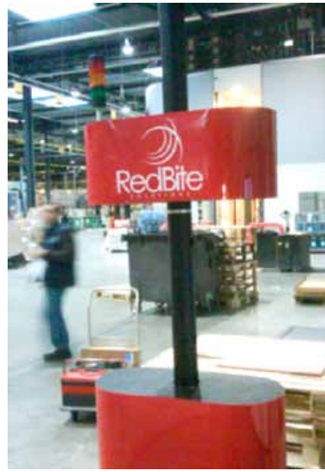
All in one solution developed for the WP10 pilot. This pillar contains antennae, reader, middleware and EPCIS repository.
